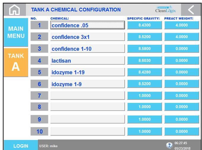
The screenshot shows the 'TANK A CHEMICAL CONFIGURATION' screen. It features a table with columns for 'NO.', 'CHEMICAL:', 'SPECIFIC GRAVITY:', and 'PRACT WEIGHT:'. The table contains 10 rows of data. The bottom status bar shows 'LOGIN', 'USER: mike', and the time '06:27:45' on '05/23/2018'.
