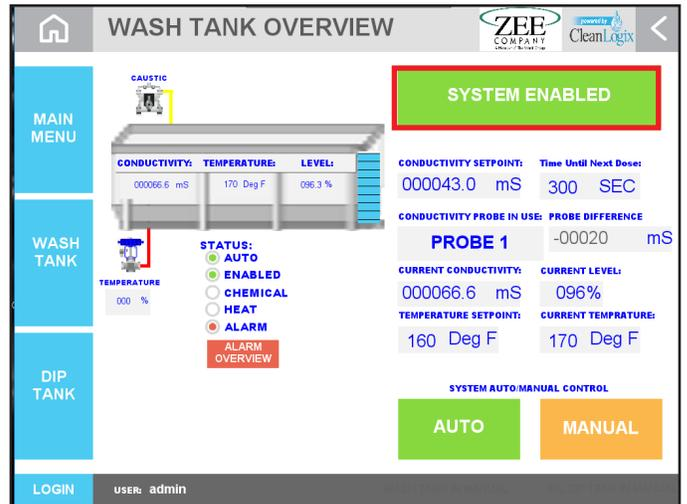
Figure 10.1: Wash Tank Overview disable system selection
