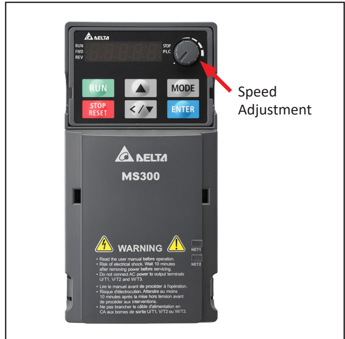
Fig. 6.1: Delta MS300 (AD GS20) Variable Frequency Drive
