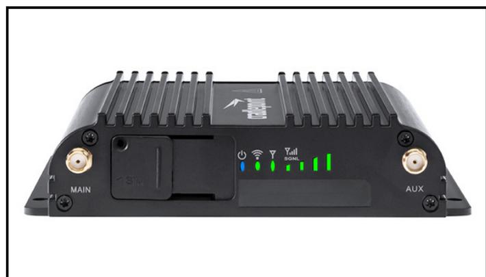
Fig. 19.3: Cradlepoint Cell Router connection status lights
