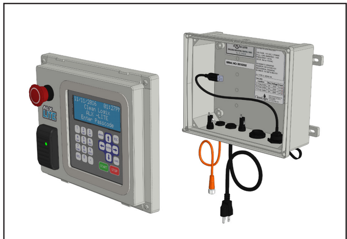
Figure 31.1: Removing enclosure cover
