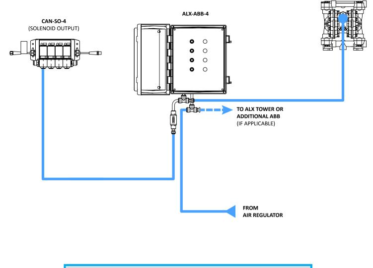
**NOTE:** Example connection shows ALX-ABB-4, installation set-up may vary.
