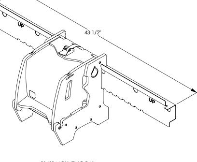
FEET INSTALLED IN WALL-MOUNT POSITION
